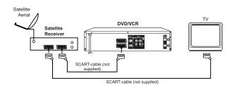
To view TV-program from Satellite Receiver, press **AUX** on the remote control of DVD/VCR repeatedly until "L1" appears on the front display.
